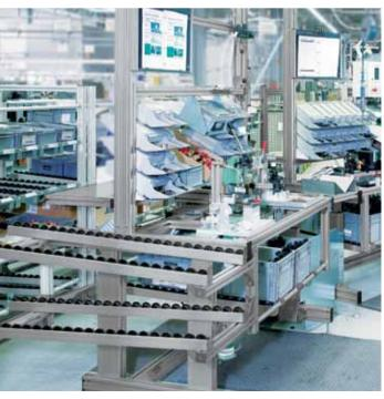
precise manner. The containers cannot slip or get swapped because the tracks are adjusted to the particular container being transported.
