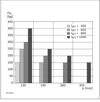
The carrying force per roller is 50 kg, and the WT must always be on at least 3 rollers. The resulting load limits for the longitudinal conveyor are illustrated in the graphic.
