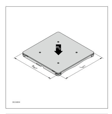
The permissible load from the conveyed goods is calculated based on the permissible WT total mass less the weight of the workpiece pallet itself including supports and special equipment etc.
