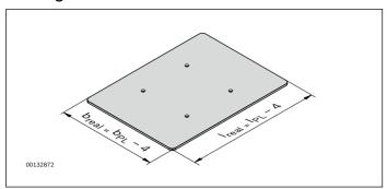
$I_{PL}$  = ordered length of the carrying plate  $b_{Pl}$  = ordered width of the carrying plate
