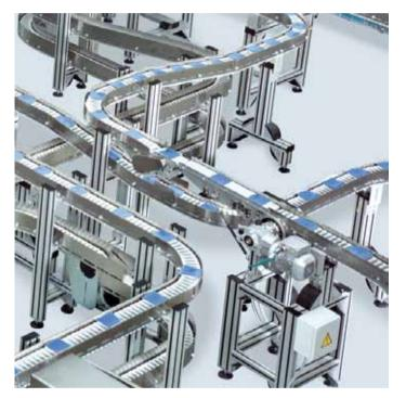
The modular Rexroth VarioFlow *plus* chain conveyor system consists of components that can be used universally for all system widths. This reduces the parts that must be stocked by the user.
