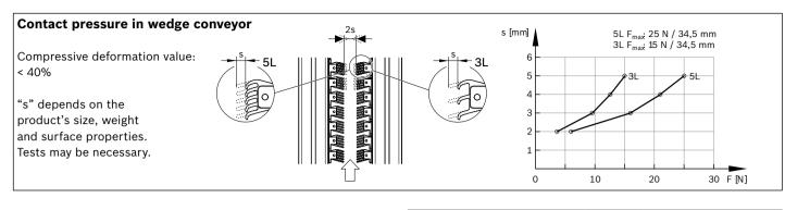
Clamping chain VF90plus 5L
