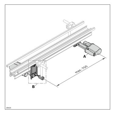
Mounting and adjustment mechanisms are placed under the conveyor system for easy accessibility of the transported material
