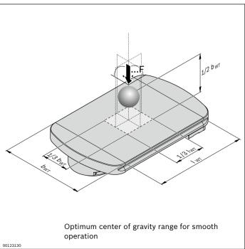
For transporting products that are not suitable for accumulation operation or are unstable due to their
