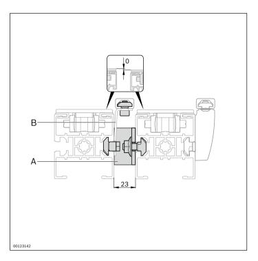
The middle lateral guide is used alternately by both sides. The section link (23 mm) (A) is used in combination with the holder for lateral guides (23 mm) (B) as a spacer between sections.
