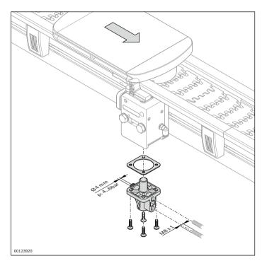
For querying the position of the stop gate via proximity switch and/or accelerating the pneumatic closing of the
