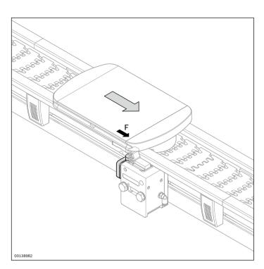
Switch bracket for a 12 mm proximity switch to install on stop gate VE 2/VF (see page 232)
