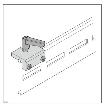
The drilling jig can be right- or left-justified and is used to drill an accurately positioned hole to secure the slide rail both on the section profile as well as on the support profile.
