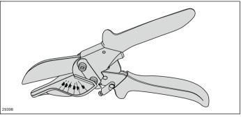
The slide rail can be easily and quickly cut to the correct length and angle with the miter cutter.
