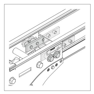
The kit enables the simple connection of the STS basic unit head, connection drive, as well as the return unit with the aluminum system.
